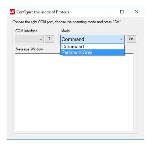
Figure 4: Windows tool to set the Proteus-II USB radio stick to peripheral only mode or command mode
