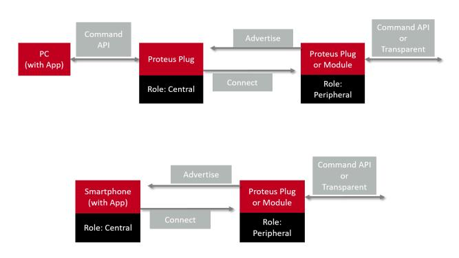
Figure 2: Typical setups for Proteus-II USB radio stick
